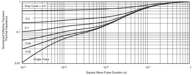
Normalized Thermal Transient Impedance, Junction-to-Foot
