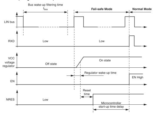
Figure 4-5. LIN Wake-up Diagram from Sleep Mode
